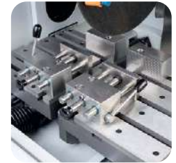
Transversal table with motorized movement Ref. 50391
