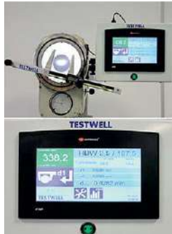
Retrofitting of hardness test machine
