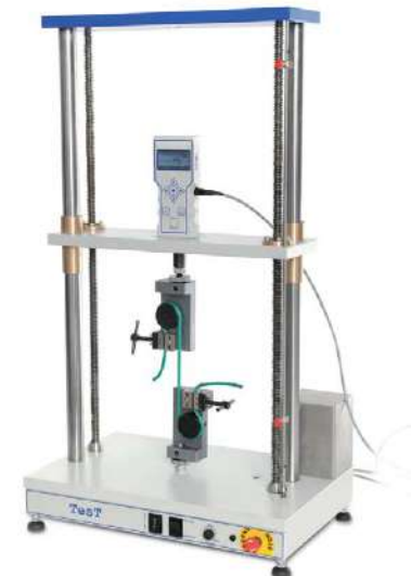
Motorized machine with force and displacement measurement
