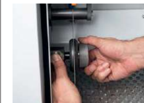
Quick-release nut for T205/T215 Tool-less cut-off wheel change Ref. 51725
