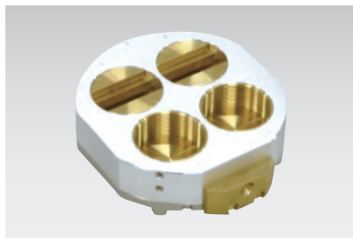
Large Specimen Holder [LH4] XM-86LH4 Maximum specimen size: 36 mm dia. × 20 mmH × 4
