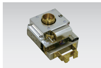
Specimen Rotation Holder XM-81450 (TRH) Maximum specimen size: 25.5 mm dia. × 15 mmH 0 to 20° tilt and endless rotation. Cable kit XM-11420 (CKMH) is required.
